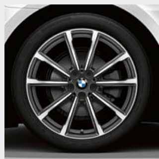
□ 19" light alloy wheels V-spoke style 685 Orbit Grey, gloss-lathed, wheel size 8.5J x 19 with 245/45 R19 tyres.
